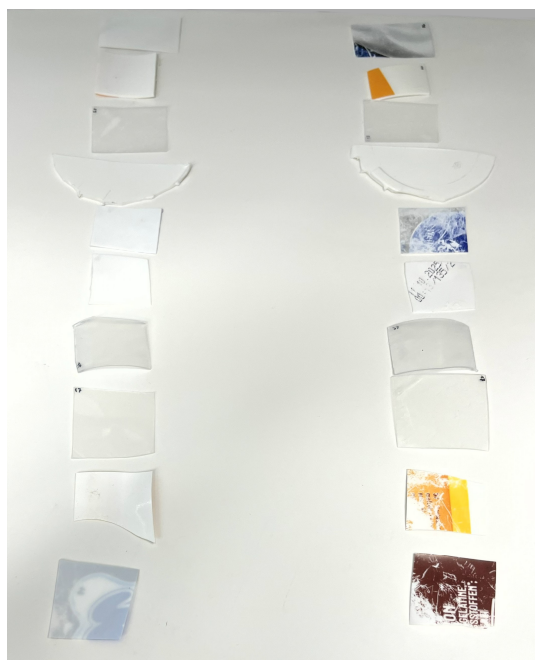
Figure 1. Depiction of 20 samples during spectral acquisition. Each sample stems from a previously collected post-consumer PP lightweight packaging. To avoid interfering spectral artifacts, detachable components were removed and samples were washed beforehand. Printed clear/white packaging was included.
